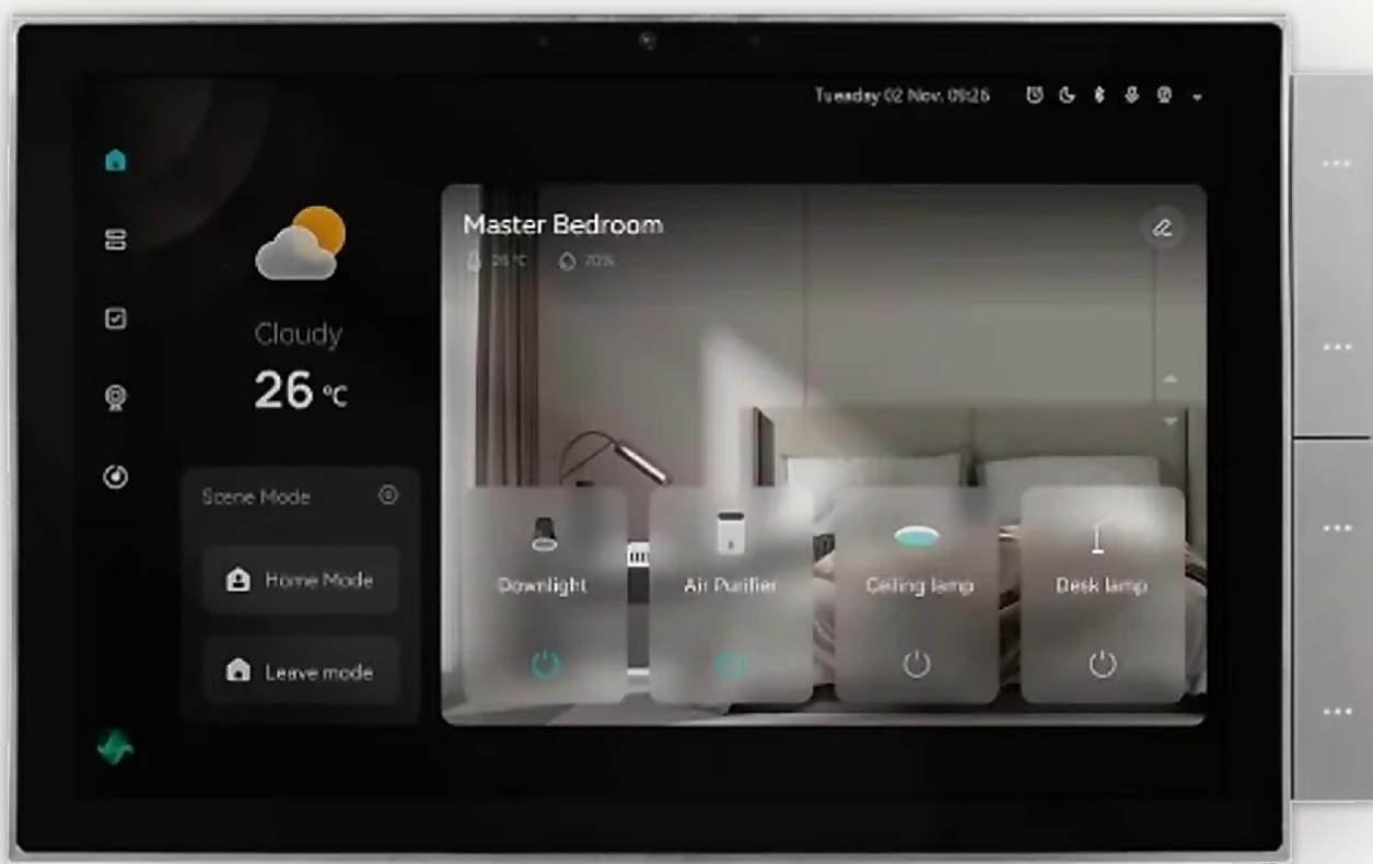
SHOWN: SPARK 10-INCH PANEL • 237.5 × 112 MM
